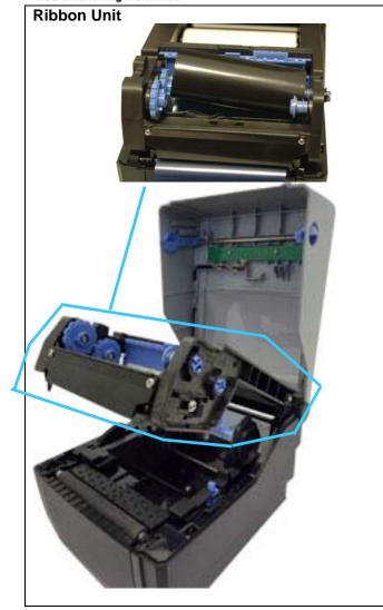
The ribbon unit serves to load the ribbon and wind up the used ribbon.
